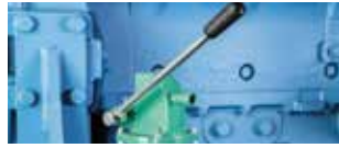
Manual lube oil drain pump
